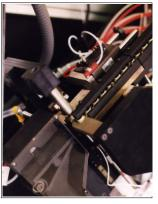
determined the threads to be good, the nut was discharged from the inspection head into a final packaging container. If the threads were defective, the nut was discharged into a rejection chute.
